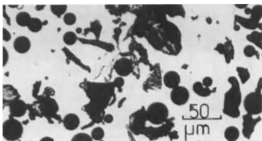
Fig.3. Microphotograph of strontium- zirconium deformed gel particles after fast extraction of anions during emulsion drops formation.
