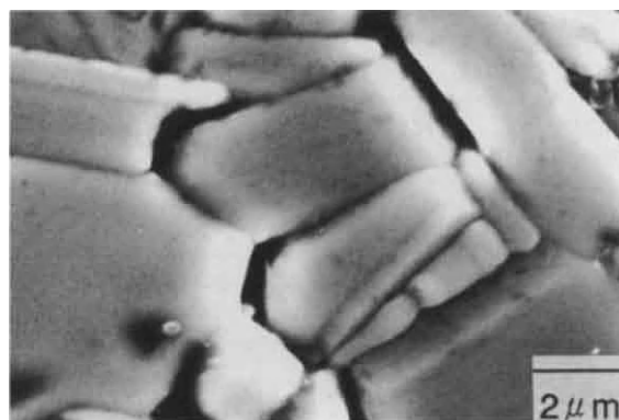
Figure 5. Microstructure of \text{Ti}_3\text{SiC}_2 deformed plastically at 1200°C.
