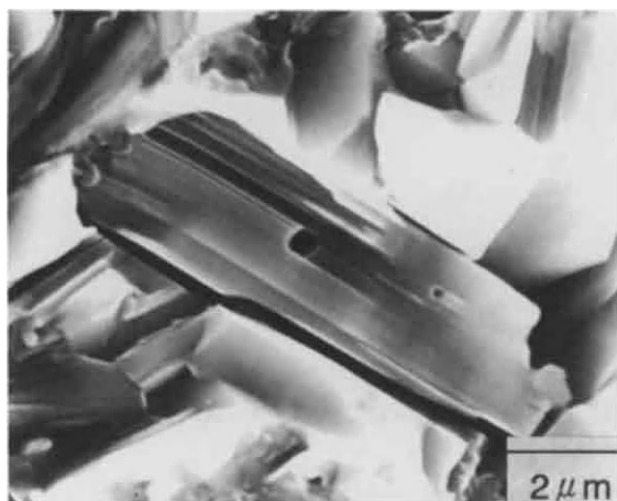
Figure 6. Fracture surface of \text{Ti}_3\text{SiC}_2 after bending test at room temperature.
