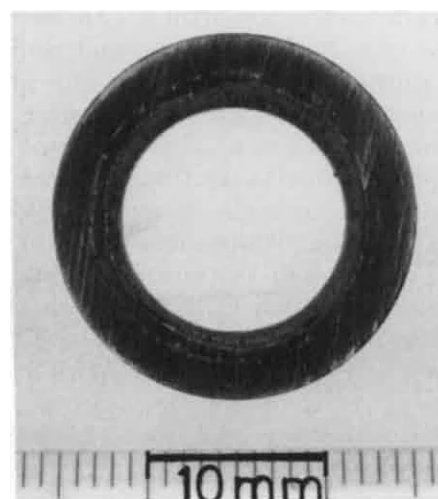
Fig. 2 Cross section of the composite pipe produced by the present C-T process under 150 G with Al-Fe 2 O 3 (including 0.5 mass % of SiO 2 ) thermite powder packed as generating 1.5 kJ/g.
