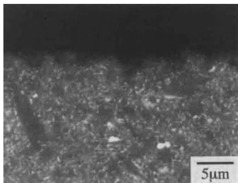
Figure 5. SEM picture of cross section of annealed specimen after corrosion test.
